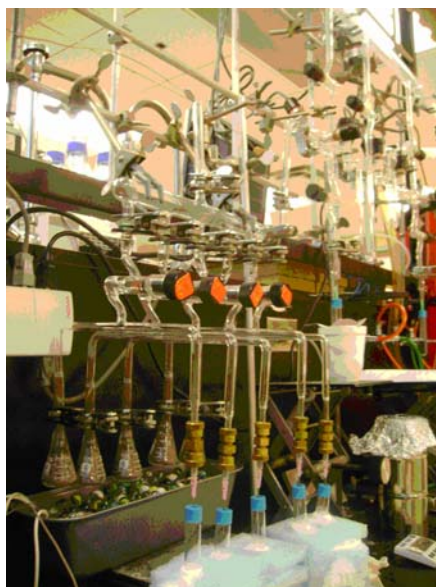
Figure 3 Distillation Line for the Vacuum Extraction of Porewaters.
