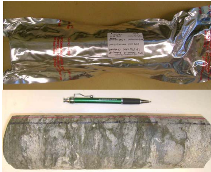
Figure 1 Vacuum Sealed Core as Received from Field. Core Sample Shown Here is ~15 cm Long
